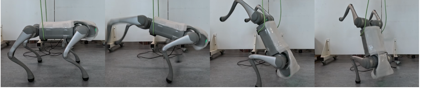
Fig. 8. Hardware deployment. Snapshots of the learned policy \pi_\theta executing a dynamic handstand on the Unitree Go2. See companion video.
